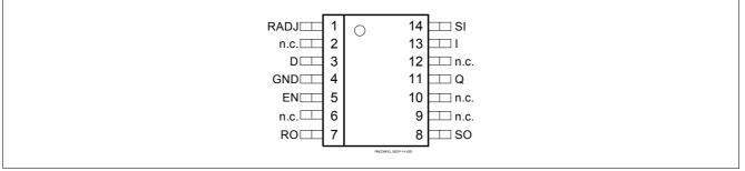
Figure 5 Pin Configuration (top view)
