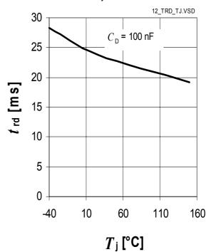
Delay Capacitor Discharge Time  $t_{\rm rr,d}$  versus Junction Temperature  $T_{\rm i}$
