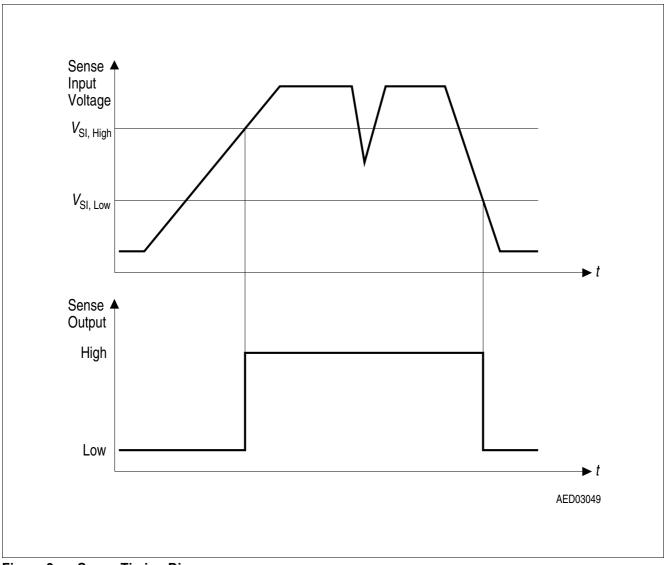
Figure 9 Sense Timing Diagram
