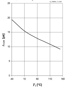
Power On Reset Delay Time  $t_{rd}$  versus Junction Temperature  $T_i$
