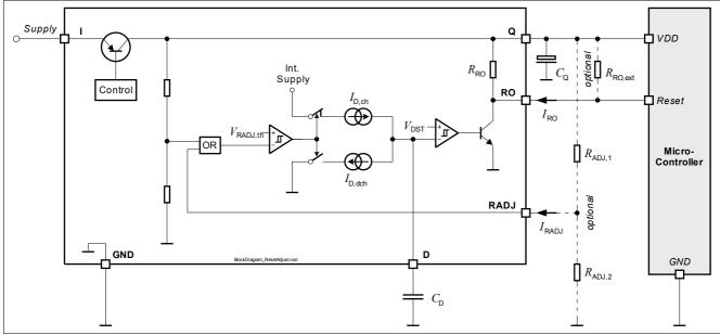
Figure 7 Block Diagram Reset Function
