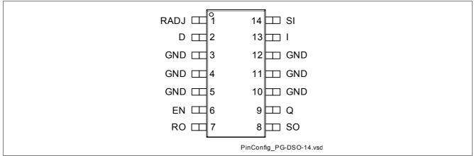
Figure 4 Pin Configuration (top view)
